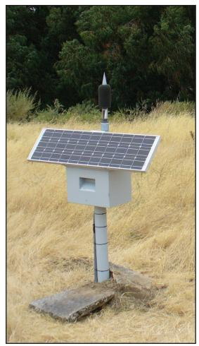
The GeoSonics/Vibra-Tech Re:mote Noise Monitoring System allows our experts to remotely monitor and record data for community noise studies. Results are collected and posted to a customized client website with an alarm notification system. These results can help address community noise issues, show relative change and establish compliance ordinance criteria for existing or new permitting process procedures.
