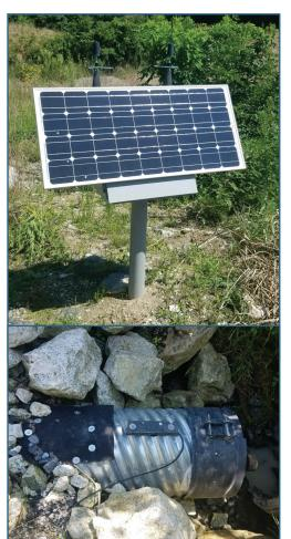
The GeoSonics/Vibra-Tech Re:mote Environmental Monitoring System can remotely monitor a variety of environmental conditions such as water levels, flow rates, pH, conductivity, turbidity, precipitation, wind speed and wind direction. And if a sensor exists to collect other environmental data, our experts can post your results to a customized client website with an alarm notification system.
