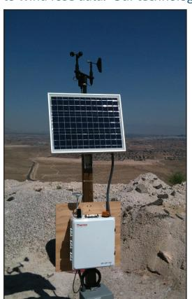
suspended particulate, PM10 or PM2.5. With our Re:mote monitoring technology, this data is collected continuously and posted to a customized client website with an alarm notification system. We have the ability to use our system as a fence line monitor, helping to understand neighbor dust complaints.
